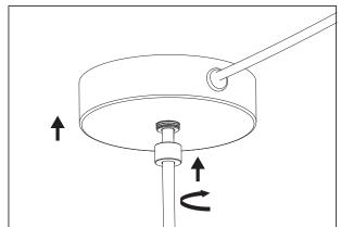
Turn the cover plate to align cable in desired direction.
