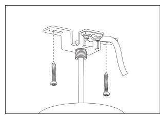
Mount the ceiling bracket to the ceiling with screws.
