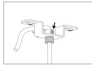
Adjust the height of the lamp by pulling the cable through the cable relief.
