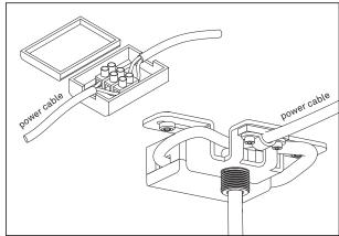
If the power cable is surface mounted make sure to put the cable through the hole in the cover plate before the following,
