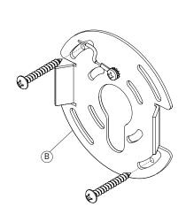
Attach (B) to your wall or ceiling using screws and plugs. Ensure the central keyhole aligns with your wall cavity.
