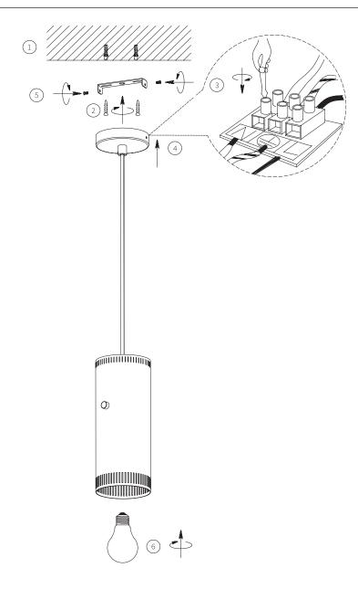
If the external flexible cable or cord of this luminaire is damaged, it shall be exclusively replaced by the manufacturer or his service agent or a similar qualified person in order to avoid hazard.
