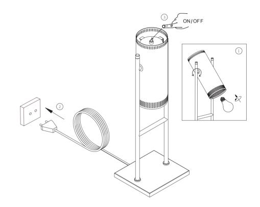
If the external flexible cable or cord of this luminaire is damaged, it shall be exclusively replaced by the manufacturer or his service agent or a similar qualified person in order to avoid hazard.
