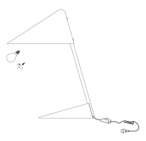
If the external flexible cable or cord of this luminaire is damaged, it shall be exclusively replaced by the manufacturer or his service agent or a similar qualified person in order to avoid hazard.
