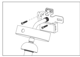
Mount the wall bracket to the wall with screws.
