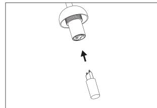
Place a G9 light bulb in the socket. The bulb is NOT included.
