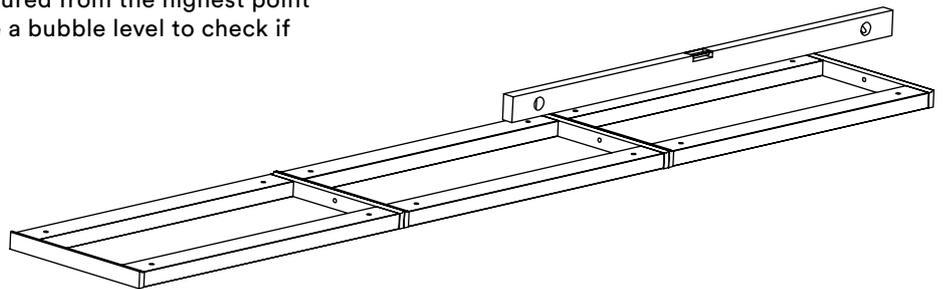
4. Afterwards level the front edge of the plinths in the same way by means of adjustable feet and the bubble level until both depth and length is 100 % leveled up.
