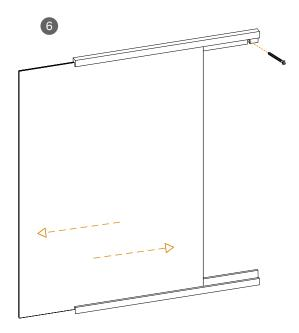
Place both the mirror and the upper list loosely on the bottom list, remember to hold it in place to prevent it from falling. Slide the mirror to both sides and screw the upper list onto the wall. Lastly, slide the mirror glass into place.
