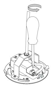
Use a pencil to mark fixing holes in the ceiling where the pendant is to be mounted. If there is a junction box in the ceiling, then the steel bracket has slots which can be used in conjunction with standard European and US junction boxes. If relevant, the input mains cable can be inserted through the centre hole in the steel bracket and passed beneath the LED driver (A). The input mains cable can also be inserted through the mousehole on the side of the plastic ceiling canopy (B), if needed.
