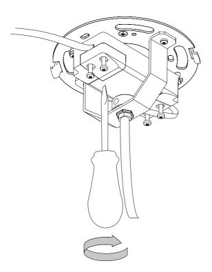
Adjust the cable from the light source, making sure that it is not pulling on the LED driver or in way of the plastic canopy. Tighten the cable grip again and make sure that the cable cannot be moved. The plastic canopy can now be replaced on the bracket.
