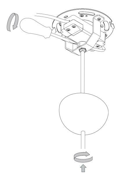
Due to the handmade manufacturing of the glass shade, some shades will have a slight difference in the distribution of weight, which can cause them to tilt slightly. If this happens, you should reposition the three supportive legs inside the shade, adjusting them until the shade is level.
