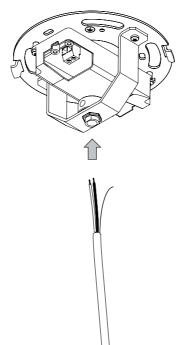
After inserting the cable through the cable grip, as shown in the previous step, locate the fibre support cable and feed it through the small hole next to the exit hole on the cable grip (1). Once the fibre support cable has exited the other side, as shown below, the smaller fixed screw on the side of the cable grip can be fastened with the provided hex key, securing the fibre support cable in place (2).
