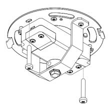
Trim the cable to the desired length, leaving 35mm of basic single insulation exposed for wiring and 3mm of exposed cable with no insulation. The cable is fitted with an internal fibre support cable for securing the weight of the glass shade. Leave approximately 50mm of the fibre support cable exposed for support.
