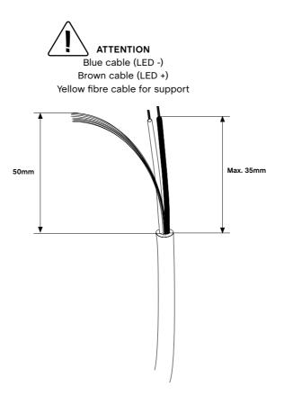
It is advised that any wire exposed with just a single basic layer of insulation is covered with the protective heat shrink provided. (Two sleeves for the basic insulated wire and one sleeve for covering the opening of the source cable). A heat gun can be used to shrink and fix this protective insulation in place (2). The double insulated mains power cable that connects to the LED driver should have a diameter between 2 x 0.75mm<sup>2</sup> - 2 x 1.5mm<sup>2</sup>.
