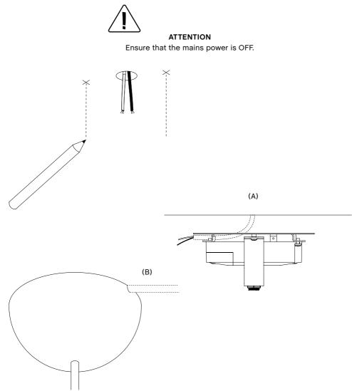
Drill holes and insert wall plugs. Ensure you use the correct type of drill and wall plug for the type of ceiling you are drilling into.
