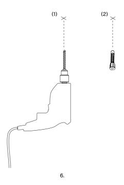
Screw the ceiling bracket to the ceiling, using the appropriate screws for the wall plugs used.
