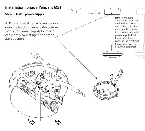
**B.** Install the power supply on the bracket by fastening the two screws.
