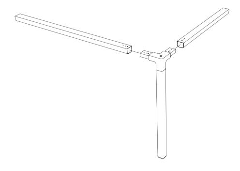
Screw 4 x L parts using the J part. Repeat this step for all 4 x E parts.
