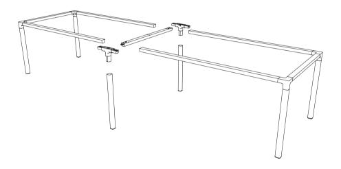
Place the M part in the F parts and tighten the bolt.
