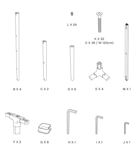
Slide the G part into the D part. Repeat this step for all 6 x D parts.
