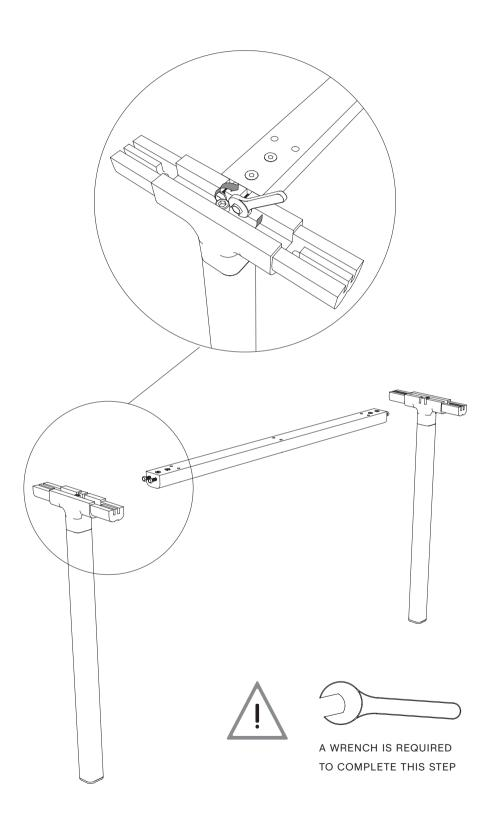
Screw 4 x L parts using the J part. Repeat this step for both F parts.
