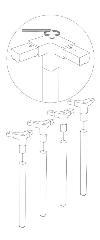
Place B and C parts into the E part. Repeat this step for all 4 x E parts.
