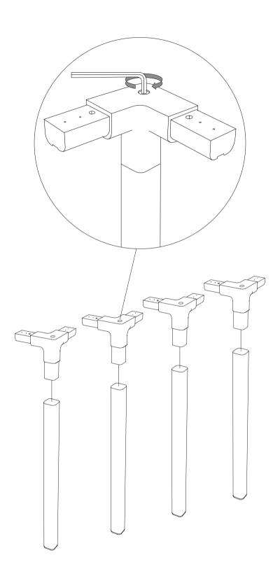
Place B and C parts into the E part. Repeat this step for all 4 x E parts.
