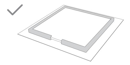
Slide the F part into the D part. Repeat this step for all 4 x D parts.
