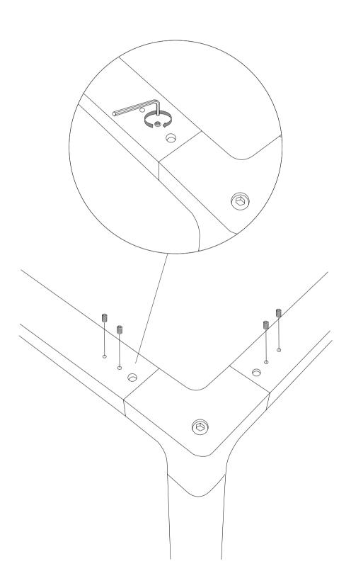
Screw the F part to the D part, using the H part.
